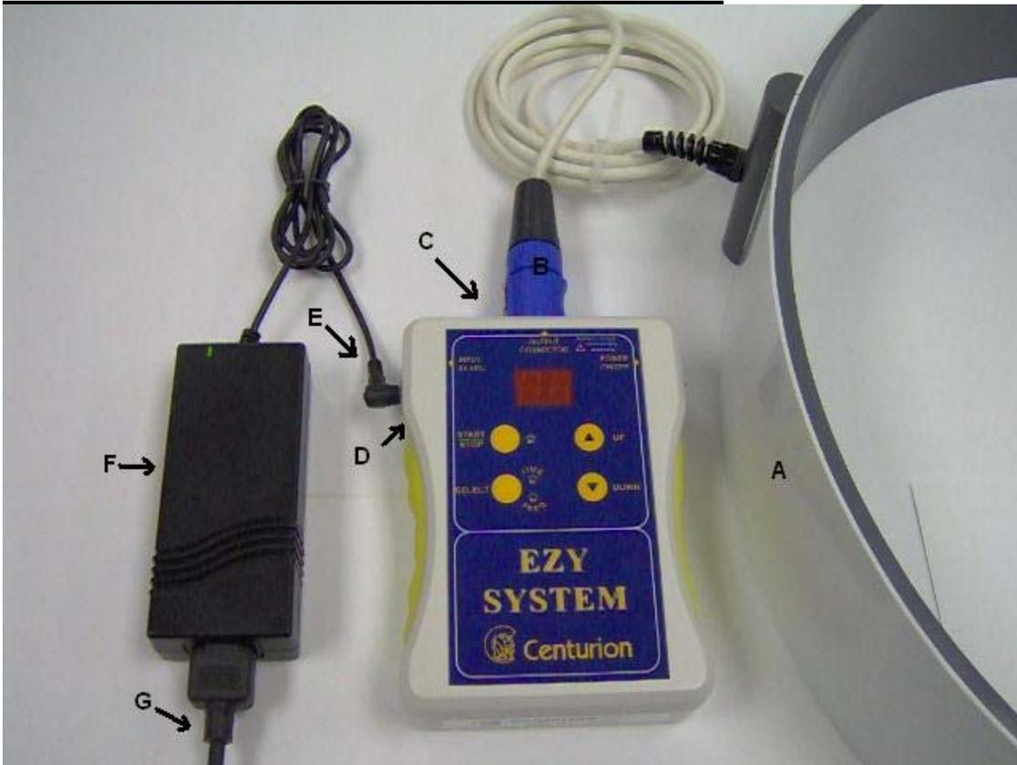
**Figure #1: The EZY System Controller, Power Adapter and Applied Part**
