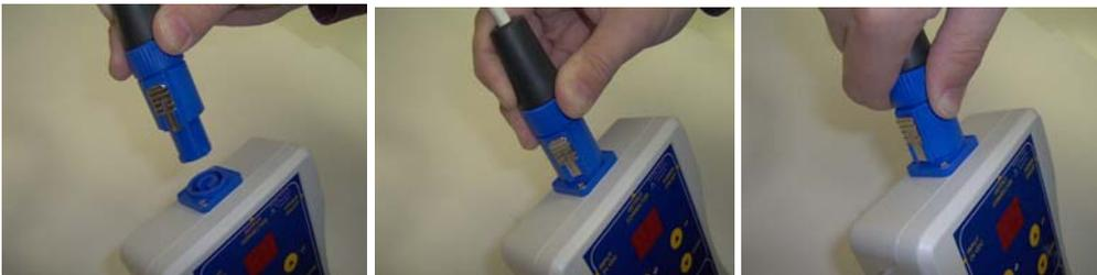
**Figure #2: Connecting Output Connector to Handheld Controller**
