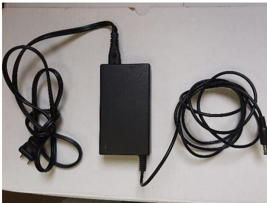
Specification; Input: 100 – 240V, 0.8 A (Max. ) 50 / 60 Hz Output: 12. 60V ===== 2.3A
